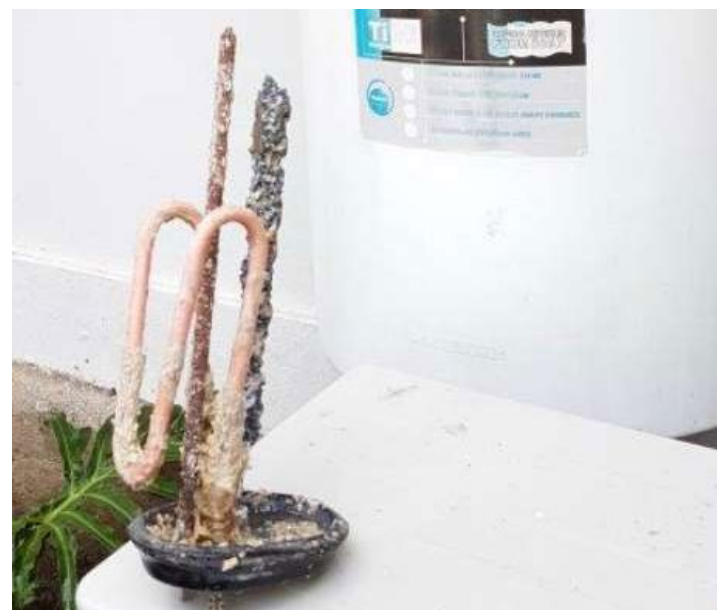
The little remaining scale is soft and easily flushed out since installation of the Vulcan Anti-Scale System.
